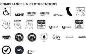
(ADA Compliant, ASME A112.18.1 Compliant, BREEAM Materials Credit, BREEAM Water Credit, CalGreen Compliant, CEC Compliant, cUPC Certified, UPC Certified, UPC Low Lead Compliant, cUPC Low Lead Compliant, EPD, Green Globes Materials & Resources Credit, Green Globes Water Credit, HPD. IAPMO, LEED Materials & Resources EPD Credit, LEED Materials & Resources HPD Credit, WaterSense Listed, NSF-61. NYC604.4, Proposition 65, Satisfies LEED Credits, TAS, WELL **Building Standard)**
