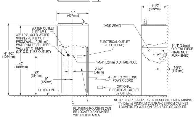
NOTE: New installations must use Ground Fault Circuit Interrupter (GFCI).
