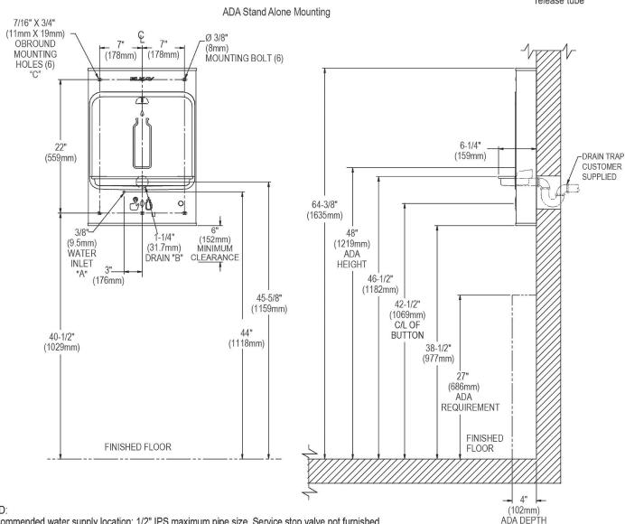
A = Recommended water supply location; 1/2" IPS maximum pipe size. Service stop valve not furnished.
